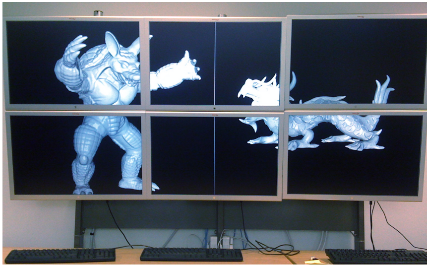
Figure 17: Display Wall using a six-Segment Canvas with a two-View Layout
