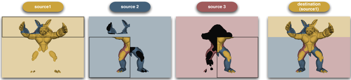
Figure 1: Sort-last rendering with direct send compositing using three channels.
