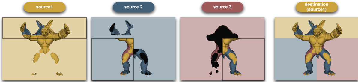
Figure 1: Sort-last rendering with direct send compositing using three channels. The first three images show the rendering buffers which contain the rendering of the partial database and the composited image of this channel. The last image shows the final, visible destination view with the fully composited image. The channels use different clear colors to identify the tile layout.
